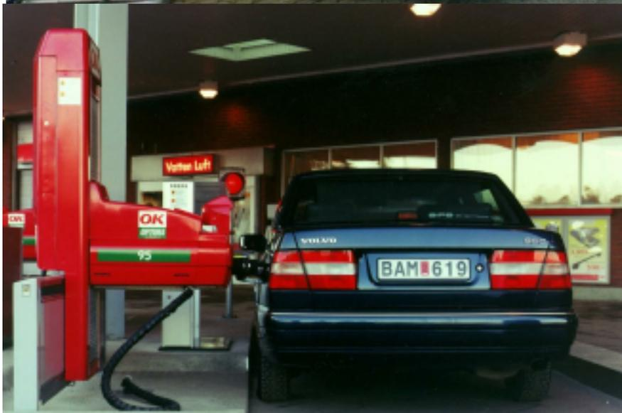
Solutions more in the line with universal design are made possible by highly specialized technology. Servolink (top) is an infrared system of warning which can draw the staff's attention to the fact that costumers at a service station need assistance to fill up. This is mainly a compensatory measure for people with disabilities. New petrol pumps with automatic filling are now being tried out (right). This solution provides the same means for everybody.
